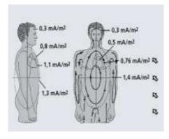
Induction of electric fields or currents in a body that is exposed to a 50 Hz magnetic field (external magnetic flux density 100  $\mu$ T). The induced current densities are greatest at the periphery and decrease within the body.
